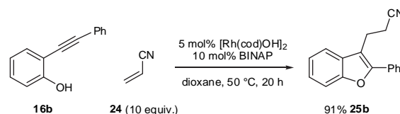
Scheme 5. Domino cycloisomerisation conjugate-addition to 24 .
